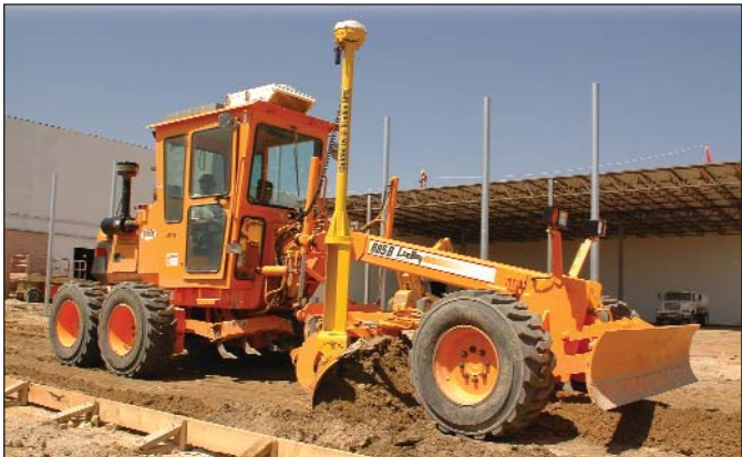
Pictured with customer-mounted Trimble GPS system
