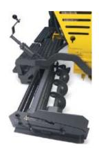
Independent hydraulically driven augers found on the screed extensions on the model 1648 Plus are efficient at moving material to the end of the extension, allowing for a "true" 13 foot paving experience.
