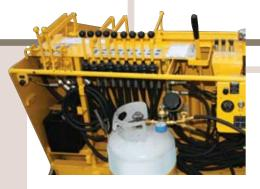
Redesigned hydraulic hose-routing system and three test ports make diagnostic access fast and clean. An engine access panel allows unobstructed access to the alternator and starter.
