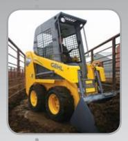
COMPACT SIZE - New, compact 1640E is as narrow as 3-feet wide\*, making it perfect for maneuvering through alleys, gates, narrow doors and corridors.
